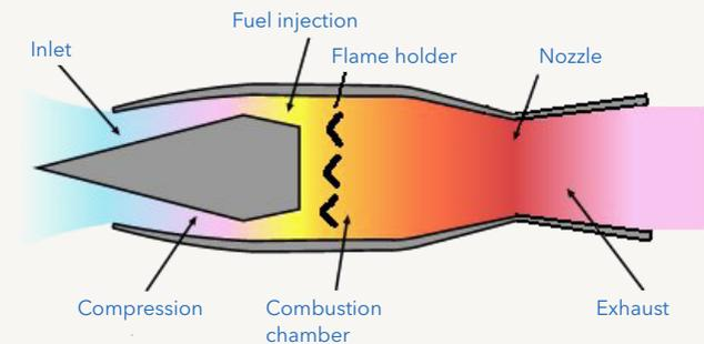
**Diagram of scramjet:** Scramjets have a different arrangement of compression, combustion, and expansion regions to ramjets, allowing air to move at supersonic speeds throughout the whole engine.
