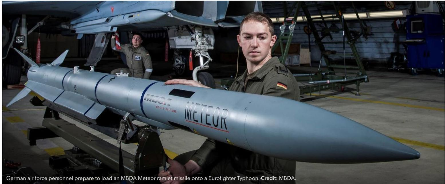
German air force personnel prepare to load an MBDA Meteor ramjet missile onto a Eurofighter Typhoon. Credit: MBDA.
