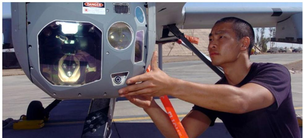
The sensor pod on a Predator drone contains sophisticated cameras, radar, and electronic tracking equipment. Credit Cohen Young, US Air Force
